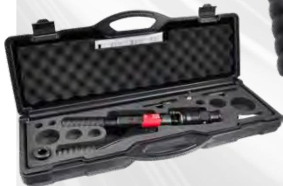
**4 INSERTI DI FORATURA TRE SPLIT INCLUSI: PG11-PG13,5-PG16-PG21**
